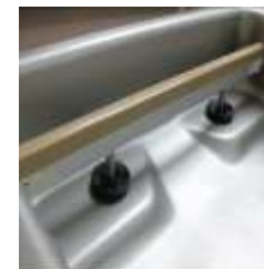
Sealing of the bar vacuum chamber
